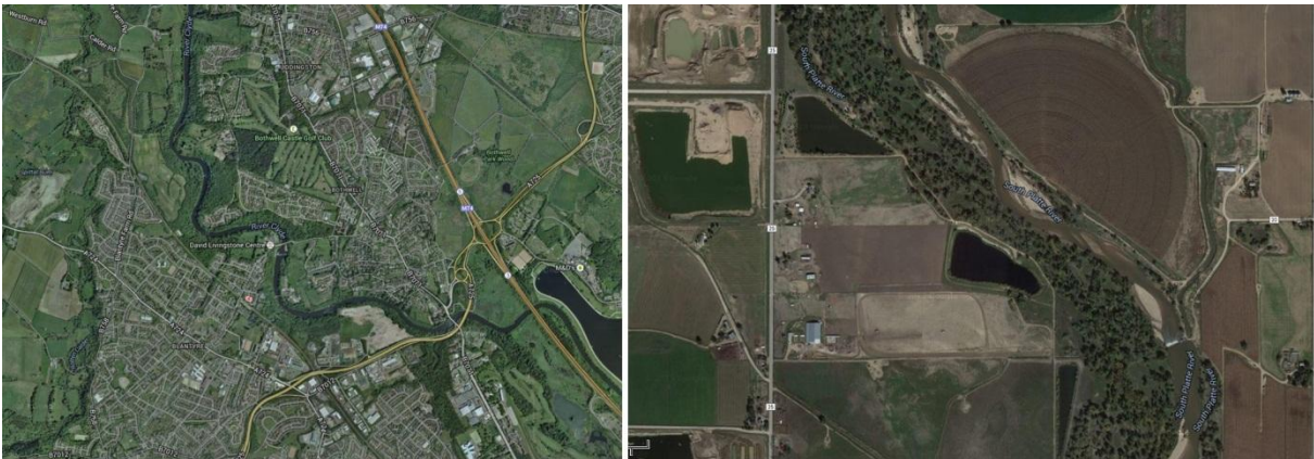
Figure 4.1. Examples of a single-thread river (Clyde, UK) and a multiple-thread river (South Platte, USA) Source: (maps.google.com)
